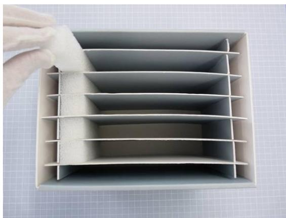
Fig 20. After assembling the partitions, the sides were filled with Ethafoam strips.
