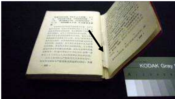
Fig. 8: tears and delamination at pages
