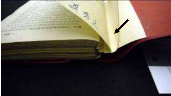
Fig. 6: plastic pulling the pages to concave shape
