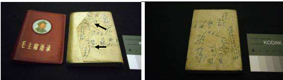
Fig. 10: pages before treatment at the left hand side; pages after humidification and flattening at the right hand side
