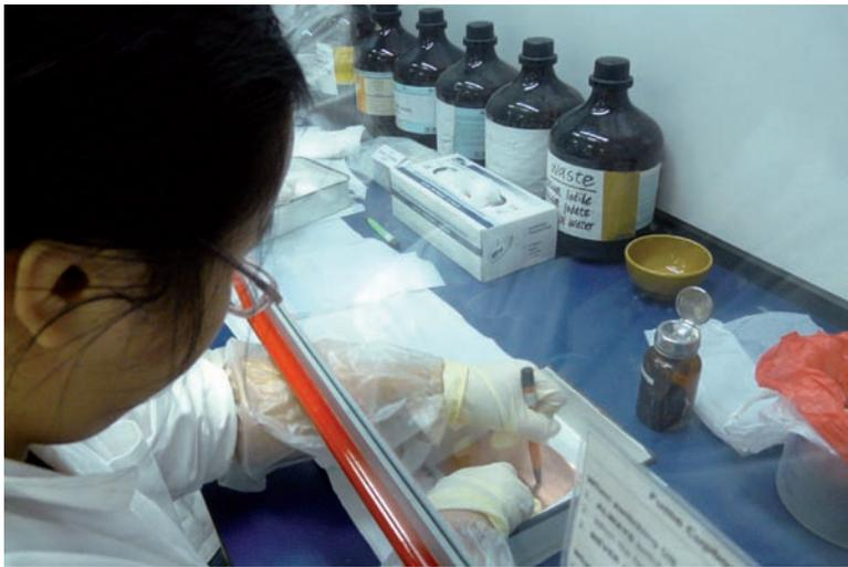
Figure 3. Preparation of the metal coupons in a fume cupboard
