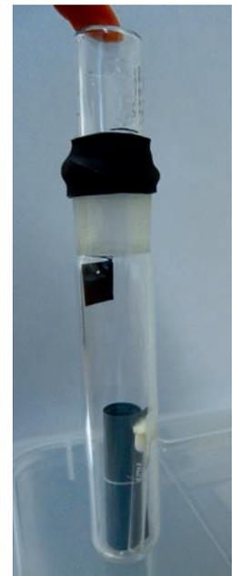
Figure 1. British Museum's ACT with one metal coupon per test tube
