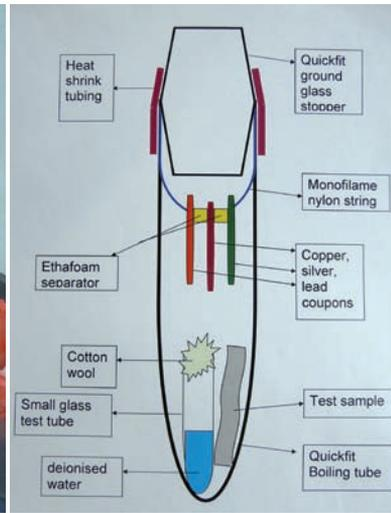
Figure 4. HCC's 3-in-1 set-up
