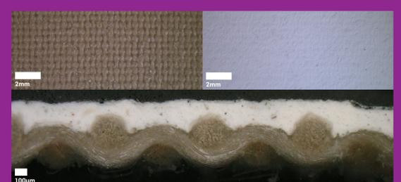
Figure 7. Sample QAG 44 — Artfix. Top left: reverse showing PET canvas plain weave (20 x 22 threads/cm). Top right: front showing priming surface. Bottom: cross section showing canvas and priming layer of PVAc (VeoVa)/acrylic (BA, MMA)/styrene with titanium white, chalk and talc, thickness 103.25µm.
