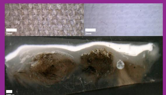
Figure 6. Sample QAG 26 — Caravaggio. Top left: reverse showing linen plain weave (11 x 12 threads/cm). Top right: front showing priming surface, micro-cracks noted in priming. Bottom: cross section showing canvas and two priming layers: top layer — acrylic (EA/EHA/EMA/MMA) with titanium white (no chalk), thickness 41.30 µm; bottom layer — styrenated acrylic (EA/MMA) with kaolinite, thickness 96.90µm.
