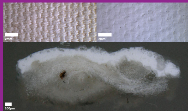
Figure 5. Sample QAG 6 — Sydney Canvas Company, 10oz cotton duck. Top left: reverse showing cotton canvas, half basket weave (11 x 30 threads/cm). Top right: front showing priming surface. Bottom: cross section showing canvas and priming layer of acrylic (BA/MMA)/PVAc with chalk and titanium white, thickness 144 µm.
