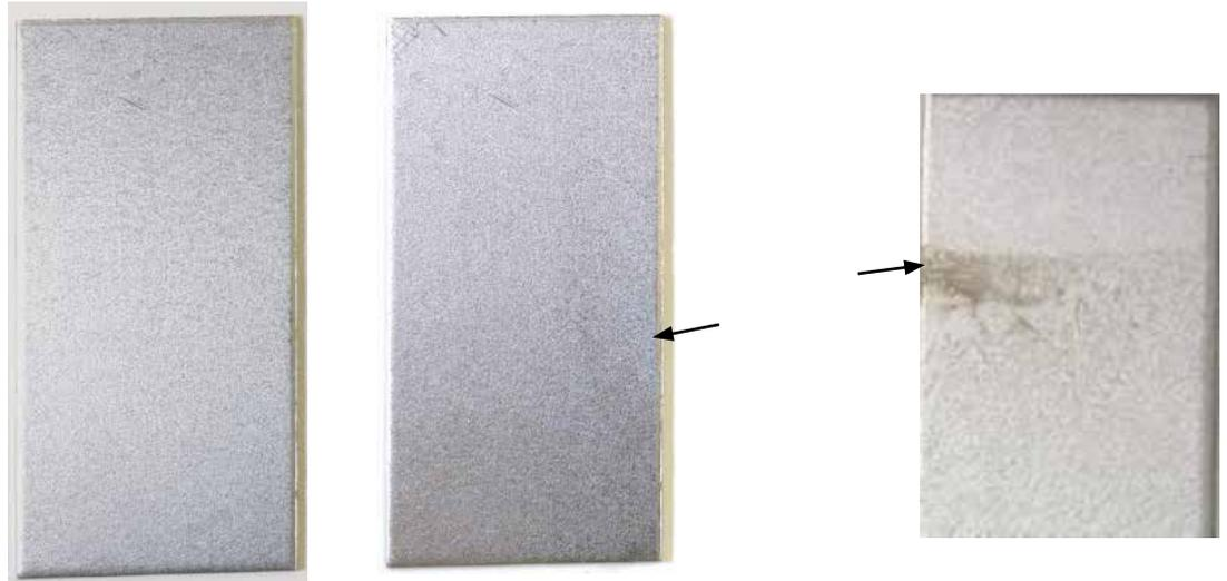
*Fig. 2. One of the coupons in U2 before waxing or cleaning (far left) and after cleaning (right), with part of a coupon from a preliminary trial (far right). The arrows indicate the locations of the brown discoloured patches that appeared during cleaning.*
