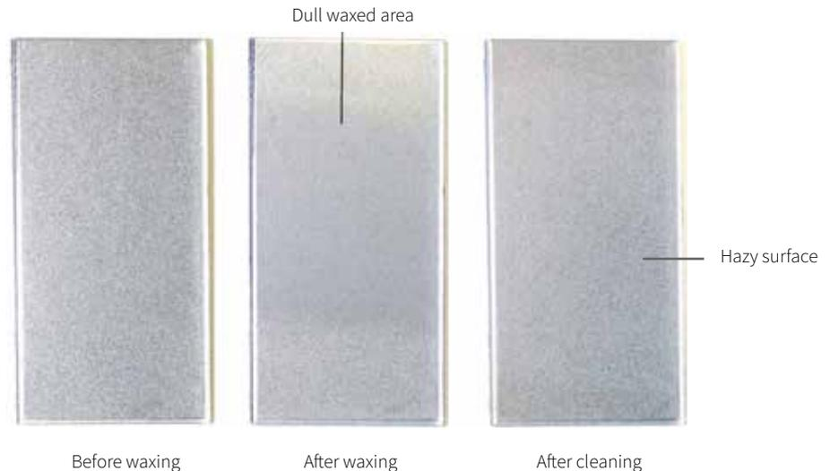
*Fig. 4. Selected coupon from U1 before waxing, after waxing, and after cleaning.*
