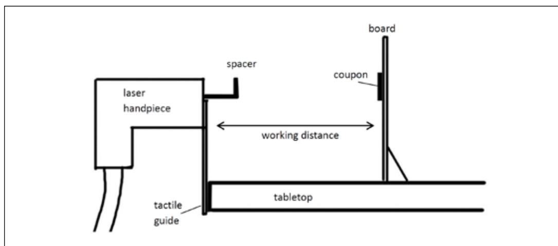
*Fig. 1. Diagram of the laser cleaning set-up used (side view).*
