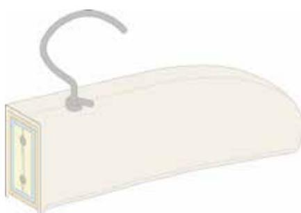
Figure 5. Diagram of a padded hanger for tops and dresses, made by a trained seamstress (Zhuo Shiya, 2019).
