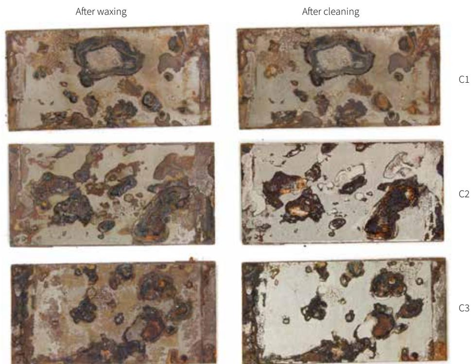
Fig. 5. Images of selected coupons in each test set, after waxing and before cleaning (left), and after cleaning (right).
