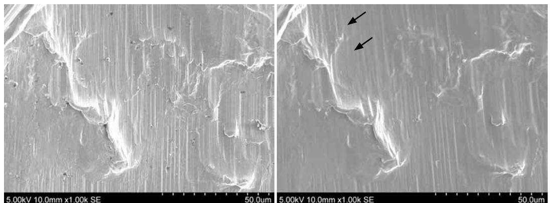
*Fig. 3. SEM image of the control coupon of U3, before laser cleaning (left) and after laser cleaning (right). A wrinkled appearance to the surface appeared in the areas indicated by the arrows.*
