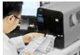
*Fig. 7. On demand printing of accession number onto RFID tag.*
