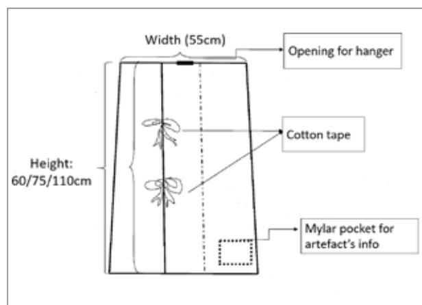
Fig. 9. Design of the dust cover for garments in hanging storage (Cheng Tan, drawing, 2012).
