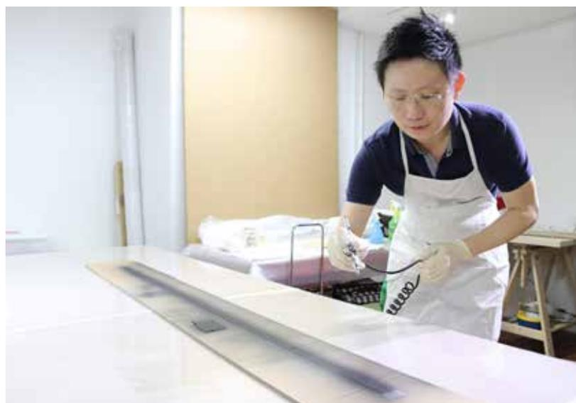
Fig. 14. Toning the Japanese paper strips using an airbrush spray.
