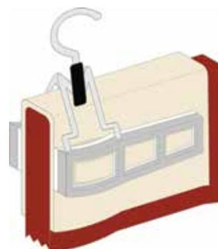
Figure 6. Diagram of a clamp hanger for skirts, shorts and pants, made by art handlers (Zhuo Shiya, 2019).
