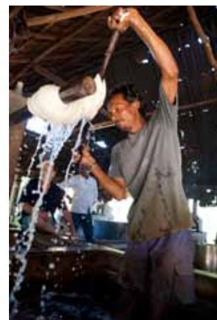
B) Washing the yarns before dyeing. The organic cotton yarns are washed before dyeing so that the threads open up and take the dye evenly.
