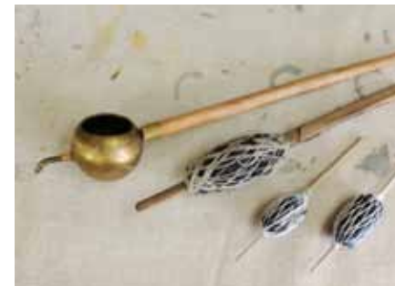
Fig. 2. Tools of the trade—traditional kalam for drawing. The kalam is made from bamboo with a bulb of hair that acts as a dye reservoir.
