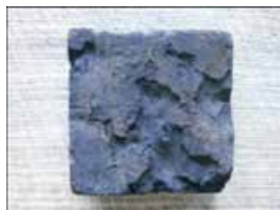
A) A piece of indigo cake used for dyeing. Blue comes from indigo. It is also used to produce, with red dye, shades of purple, or with yellow, shades of green.
