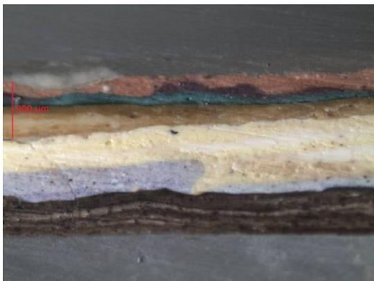
Fig 3: Cross section of pink sample of paint from *Landscape*, showing succession of many layers of paint underneath
